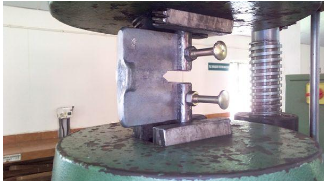
Fig -2: Standard Test piece being tested in Universal Testing Machine
