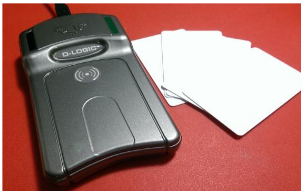
Fig 1: RFID reader and passive tags from D-Logic (Device used in this application)
