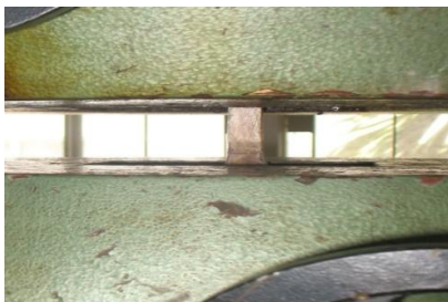
Fig -2: Tensile specimen in UTM
