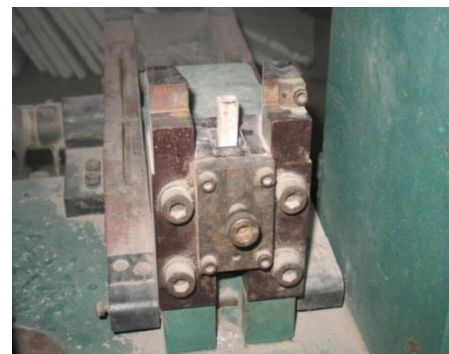
Fig -4: Impact testing of the specimen
