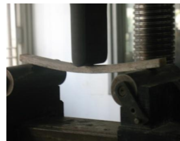
Fig -3: Flexural test arrangement
