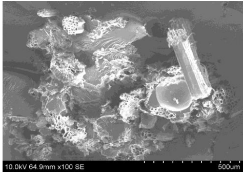
Fig -5: Untreated SEM image (x500) of banana fiber epoxy composite
