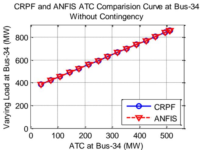
**Fig. 13** CRPF and ANFIS ATC Plot for increasing Load at Bus-34 without Contingency
