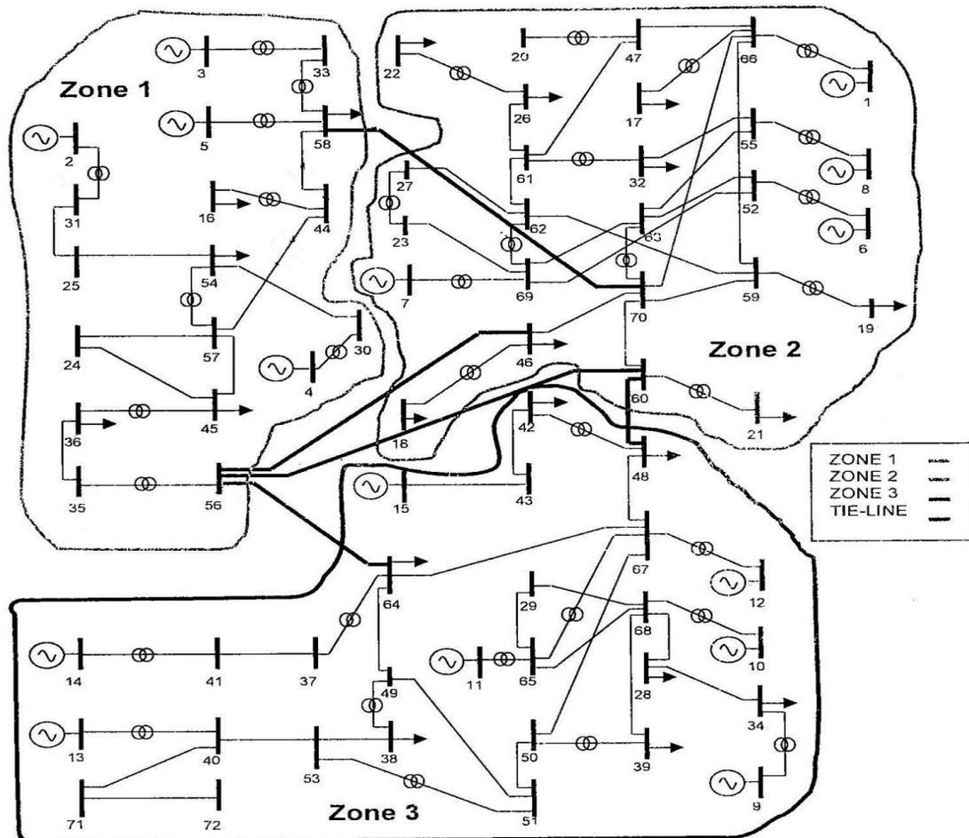
Fig. 2 Single Line Diagram of SREHV 72-Bus Test System
