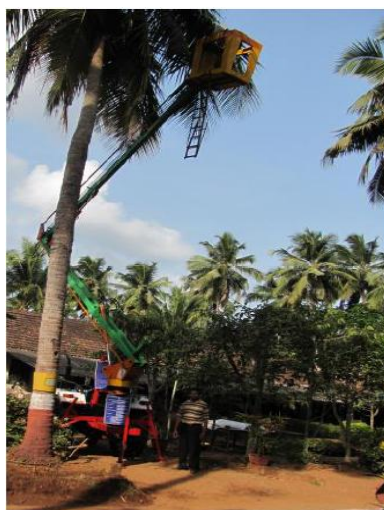
Fig. 1 Tractor mounted and self propelled coconut climber for coconut harvesting
