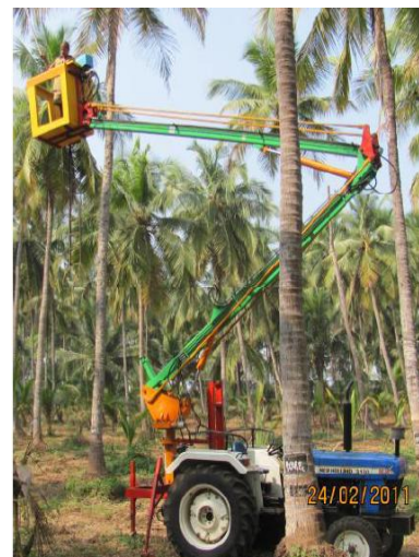
Fig. 1 Tractor mounted and self propelled coconut climber for coconut harvesting
