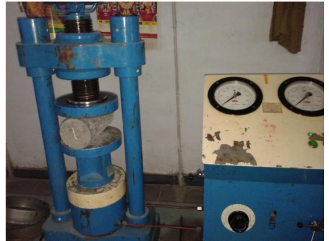
Fig 6: compressive testing machine, split tensile test for cylinders
