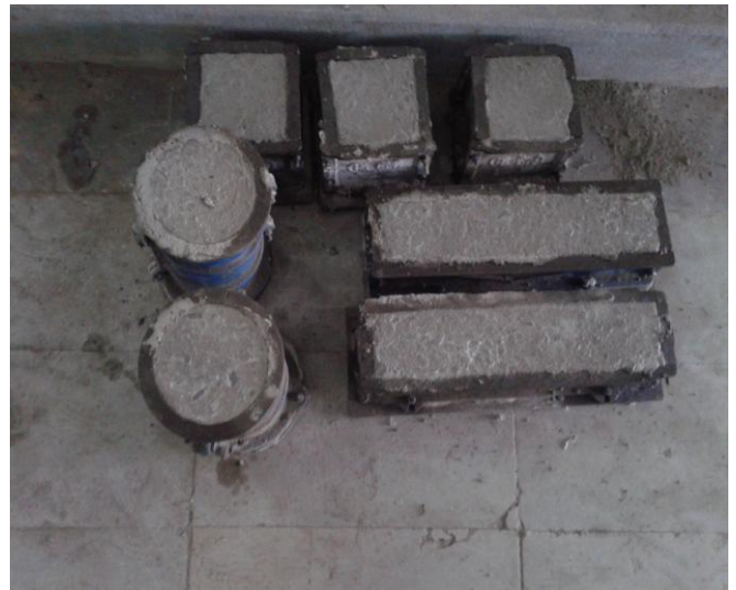
Fig -3: casting of specimens, (cubes, cylinders and beams)
