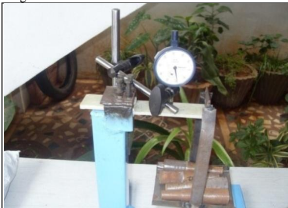
Fig 4.2: Experimental setup for deflection test.
