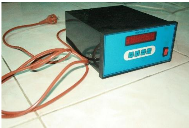
Fig 3.3: Signal Conditioning System for the Voltage Output from the Load Cell
