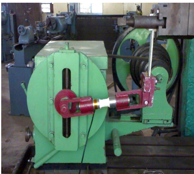
Fig 3.5: The Eccentric Mechanism to converts the rotary motion of the head-stock into translator motion
