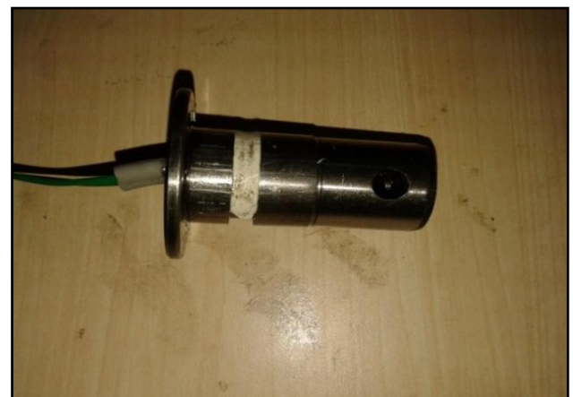
Fig -4: Mounting of strain gauge on pin
