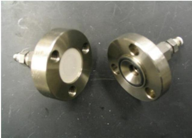
**Fig-1:** Permeation cell used for Flat membranes
