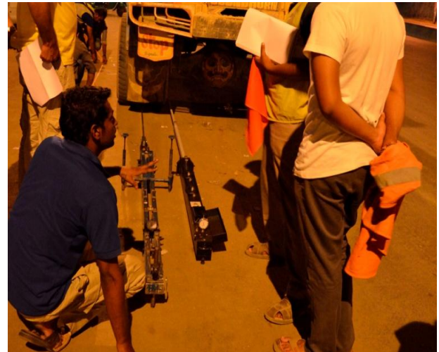
Fig2: Two BBDs is used to test on white topping.
