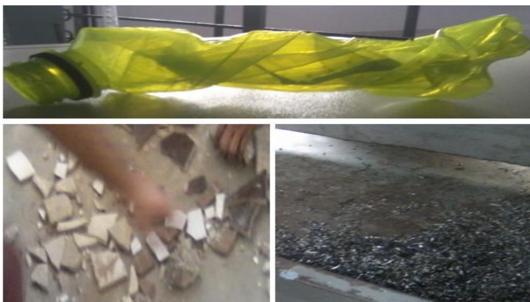
Fig 1 Constituents of manufactured aggregates-PET bottle, Ceramic waste & Lathe waste.
