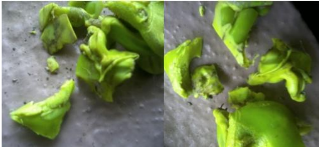
Fig 2 Manufactured aggregates using plastic as a binder.
