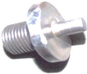
Fig 2 Tool for Ultrasonic Machine
