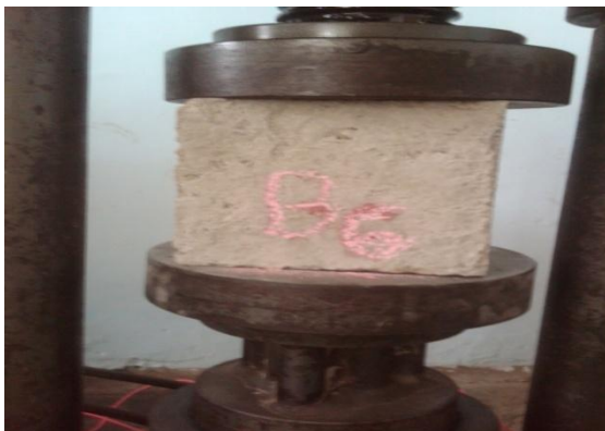
Fig. 6 testing of FRC cubes
