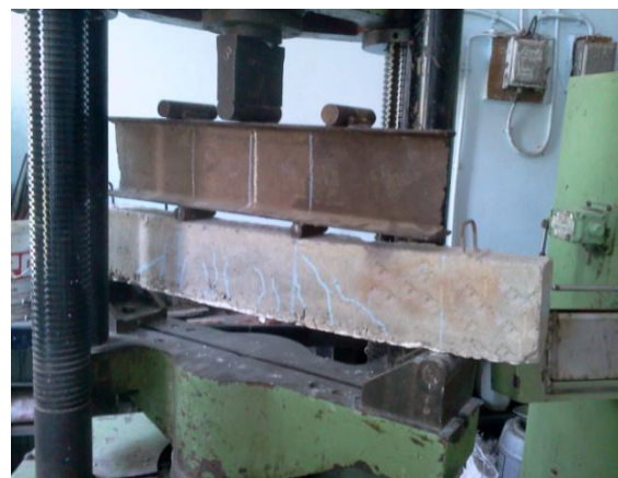
Fig. 5 cracking pattern for the control beam
