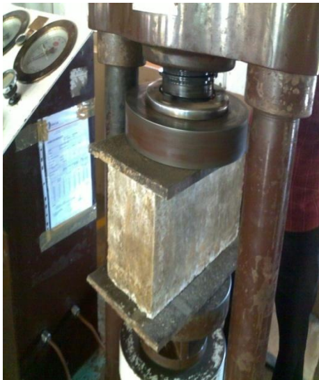
Fig -5 : Testing of Geo-polymer block
