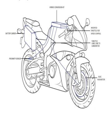
The Hybrid Conversion kit can be mounted on top of the fuel tank. In stock motorcycles, the engine is controlled by a throttle cable attached to the hand twist throttle. But once the vehicle is converted into a hybrid vehicle, we need to control a BLDC hub motor along with the engine, therefore we have to replace the twist throttle with a twist variable resistance pot.
