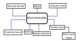
The BLDC motor and the microcontroller can be powered by using 4 12V batteries capable of providing 7Ah.
