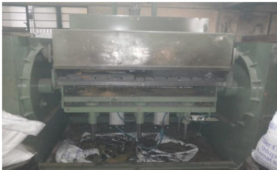
Fig.1. Shell Mould Manufacturing Machine
