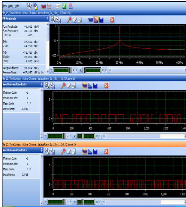
Fig 19: 30.1 MHz modulated input with recovered data pattern
