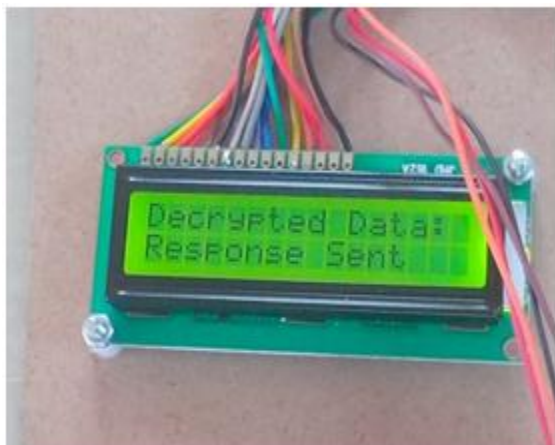
Fig 10: LCD shows receiver response
