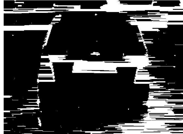
(b) Closing Operation with Horizontal SE to connect the characters present in the License Plate
