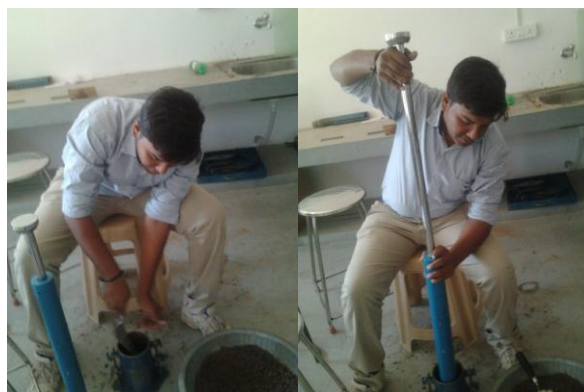
Fig 12: Moulding soil by five layer at 25 blows at each layer
