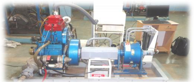
Fig.3. Test Engine -VCR Research Gasoline Engine Set-up
