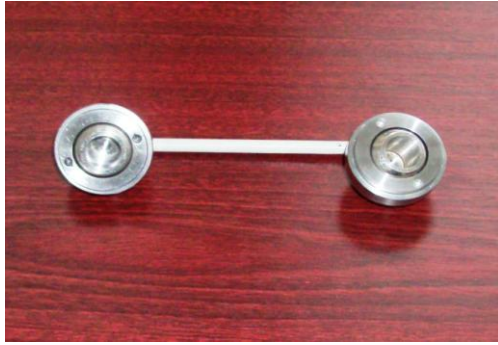
Fig 3 - Acetabular double piece (pos. 9 in figure 2).
