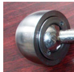
Fig 7. Acetabular cup - femoral head joint with balls in self directed movement (SDBJ).
