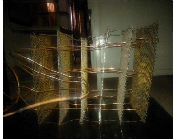
Fig.2 Condenser (side view)
