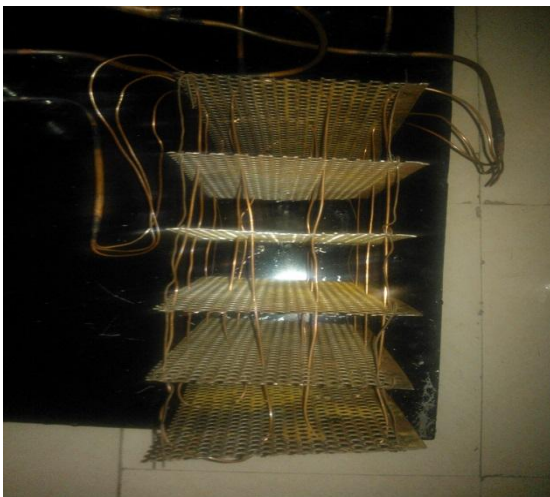
Fig.1 Condenser ( top view)
