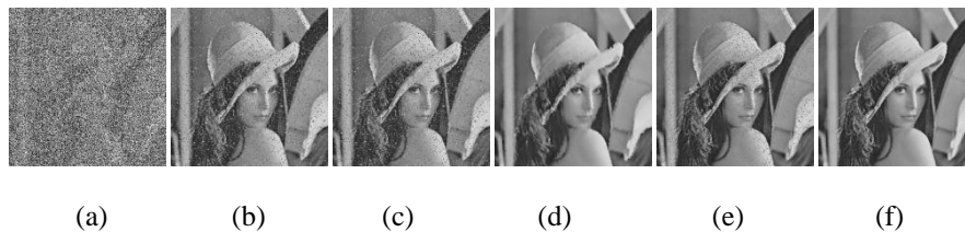
Fig-3.4: result for lena image of size 512x512 at 80% noise density (a) noisy image (b) MDBUTMF output (c) UTMF output (d) MDBMMF output (e) MMF output (f) IUTMMF output
