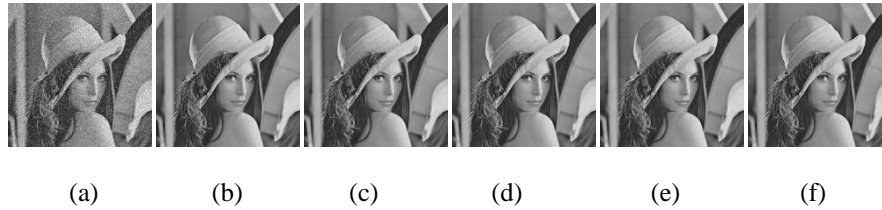
Fig-3.2: result for lena image of size 512x512 at 10% noise density (a) noisy image (b) MDBUTMF output (c) UTMF output (d) MDBMMF output (e) MMF output (f) IUTMMF output
