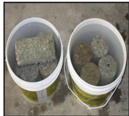
Fig 1: Water Absorption of Cylinders
