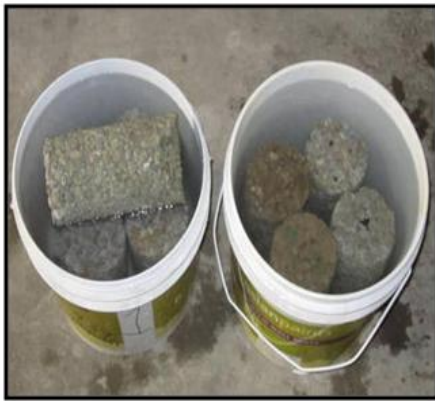
Fig 2: Cylinders Immersed in Sodium Chloride (NaCl) Solution
