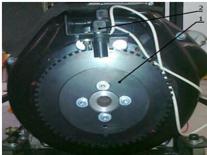
Fig -2: Location of the induction sensor for TDC 1 – one cog wheel; 2 – induction sensor.
