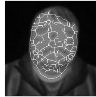
Fig. 6 Illustrative thermal template overlaid on the thermal image of the subject
