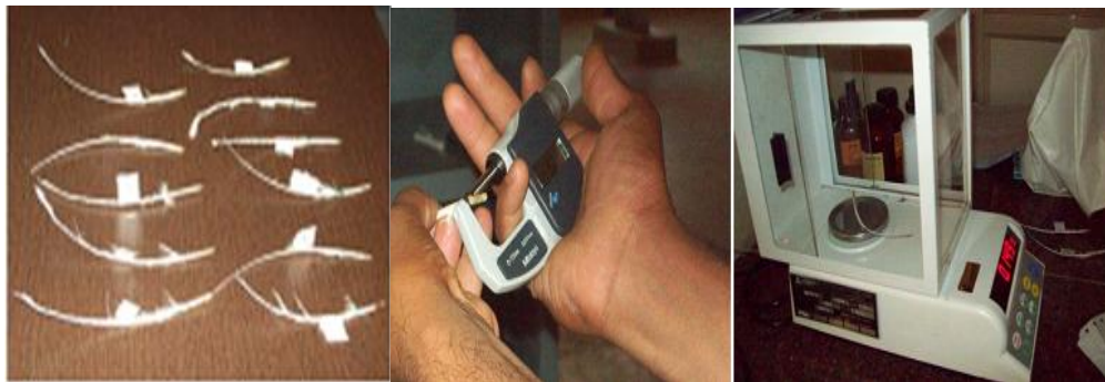
Fig A-3 Quill after stripping barbs used for weight and dimension analysis
