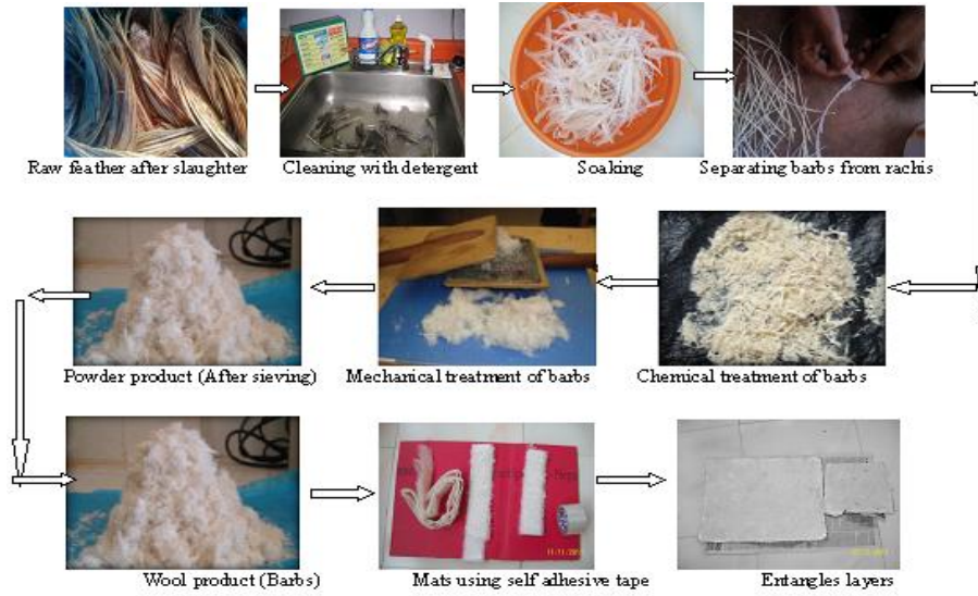
Fig A-1 Flow sheet representing the various treatments of raw poultry feathers to mat
