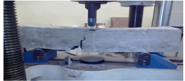
Fig -5: Bamboo Reinforcement Failed Test Specimen-A
