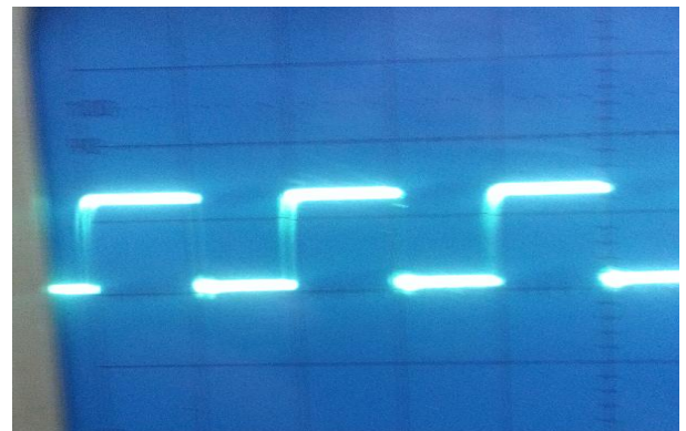
Fig-5 , PWM Signal with 50% Duty Ratio.
