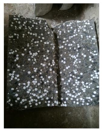
Fig. 2: Broken surfaces of failed cylinders
