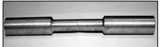
Fig-5: Photograph image of the tensile test specimen
