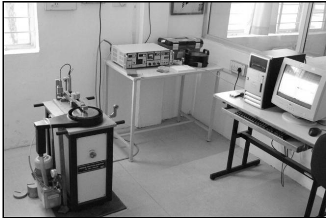
Fig-7: Friction and wear testing setup
