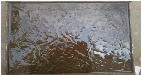
Fig-2: Preparation of laminates
