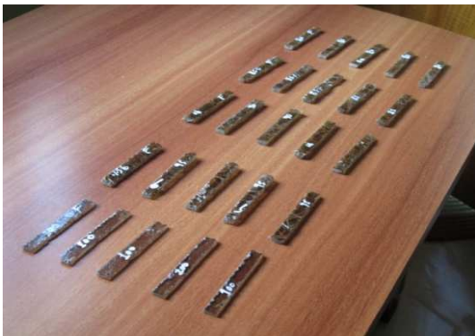
Fig- 3: Prepared Flexural specimens
