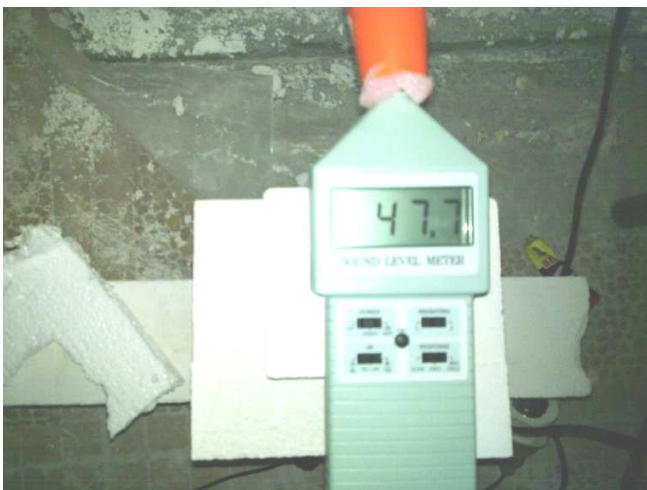
Fig--13: Measured sound from the outside of AAC panel by sound level meter
