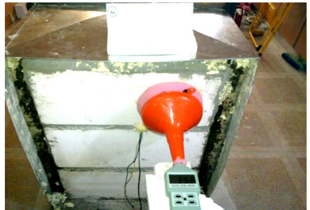
Fig-3: Sound level measuring test process
