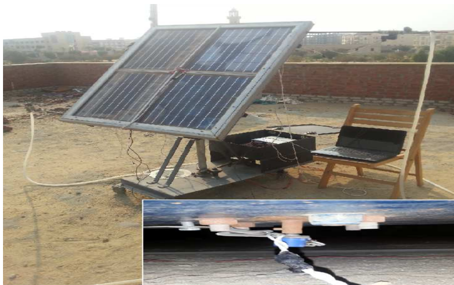
Fig (4): Place of Potentiometer to control the PV thermal system.
