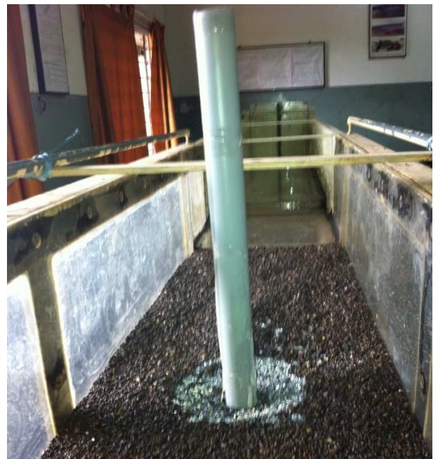
Fig.7: Pattern of scour observed around 25mm diameter pier
