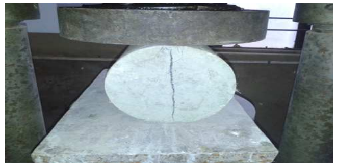
Fig 4 Tensile strength test for PFRC Cylinder
