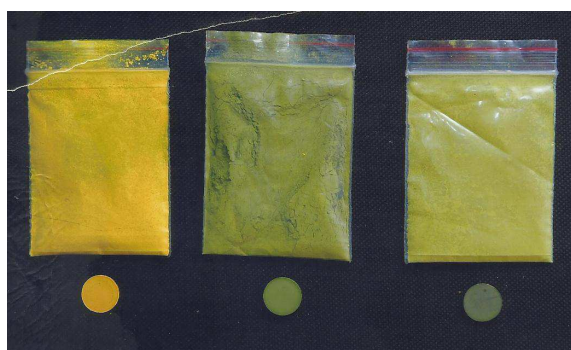
Fig. 1 :Samples produced: From the left (i) Pure CdS (ii) CdS doped with 5 wt % \text{Pb}^{2+} (iii) CdS doped with 10 wt % \text{Pb}^{2+}
