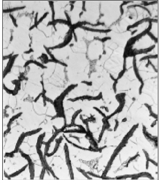
Fig-4: Optical micrograph of gray cast iron with 500x magnification: the dark graphite flakes are embedded in \alpha -ferrite matrix [18].
