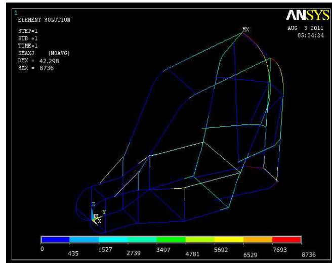
Fig. 10: Vonmises stress plot
