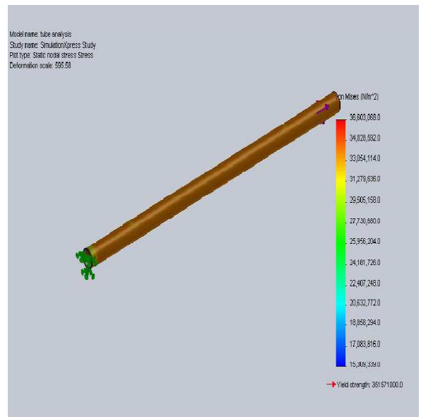
Fig-3 Tensile von-mises stress for selected pipe
