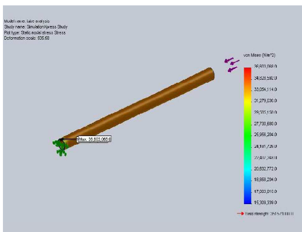
Fig2 Compression von-mises stress for selected pipe
