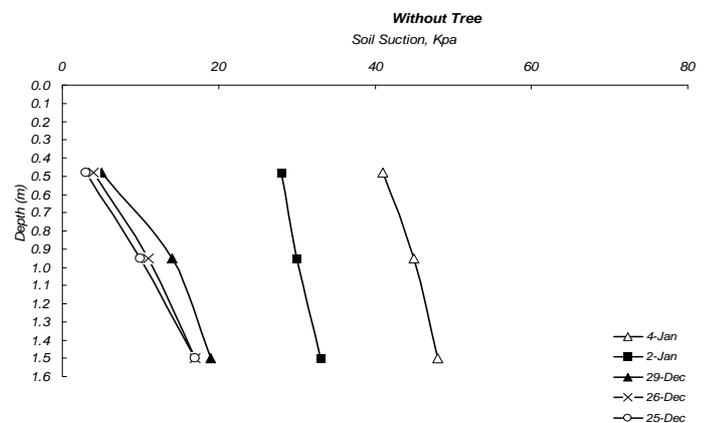
**Fig -11:** Field matric suction profile at slope without tree.
