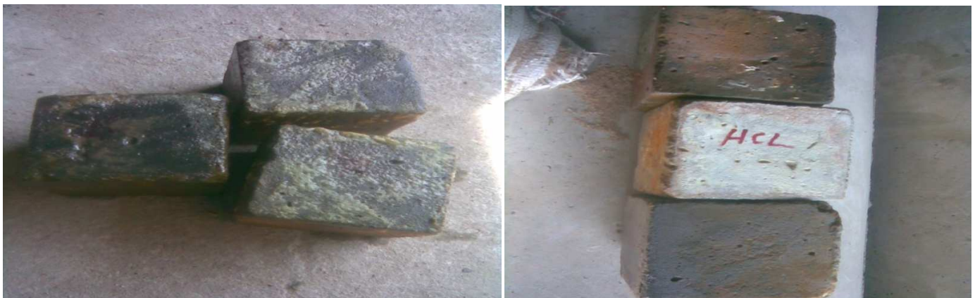
Fig 1 Test Specimens of High Strength SCC mix of M100 grade immersed in HCL solution
