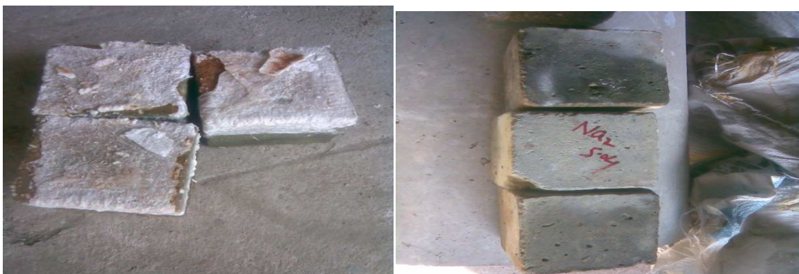
Fig 2 Test Specimens of High Strength SCC mix of M100 grade immersed in Na 2 SO 4 solution
