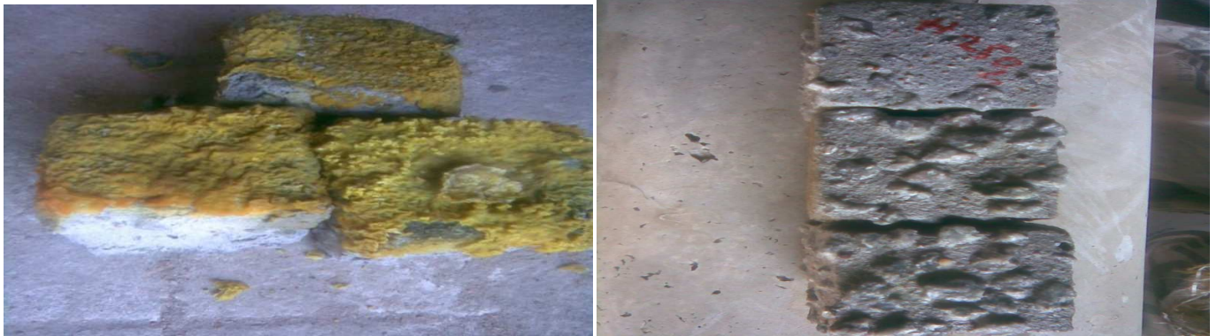
Fig 3 Test Specimens of High Strength SCC mix of M100 grade immersed in H 2 SO 4 solution
