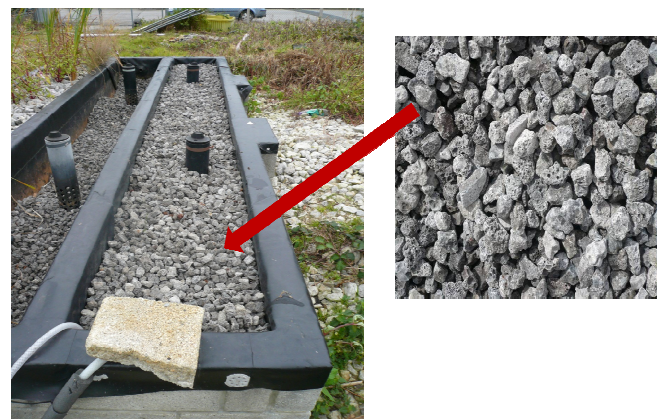
Figure1. The subsurface horizontal-flow Blast-Furnace Slag Filter (left); blast furnace slag (right)
