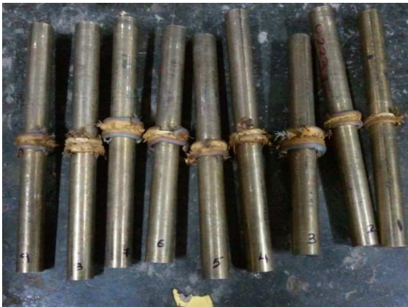
Fig 3: Specimens after Welding
