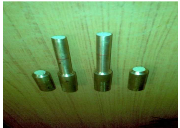
Fig 4: Run 3 and Run 4 braked at the neck portion
