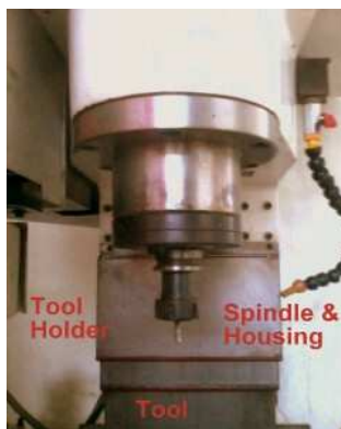
Fig-1: Schematic of end-mill spindle unit
