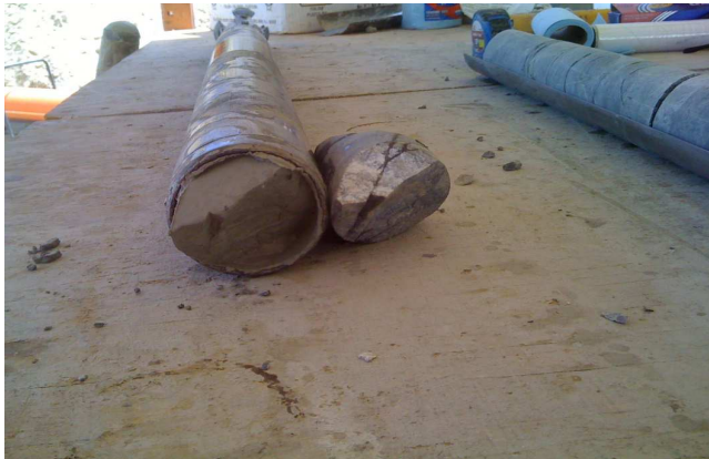
Figure 4: Determining top of hole marking by matching true orientation
