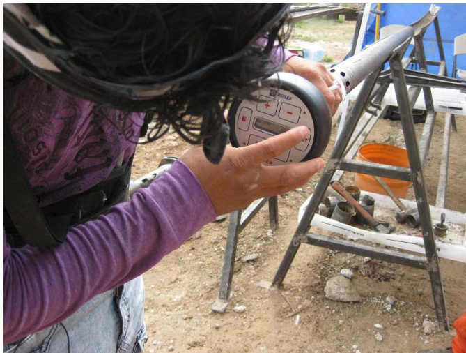
Figure 8: Using the Reflex ACT II tool to find orientation and reset timer
