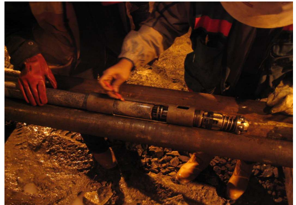
Figure 6: Transferring orientation to rock core using Ezy-Mark system
