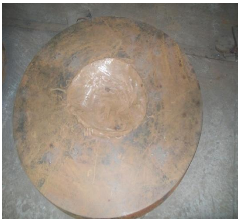
(Failed Blanking Plate)
