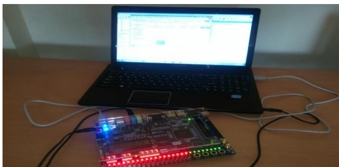
Fig-13: FPGA Implementation of audio signals using Cyclone 4 Hardware.
