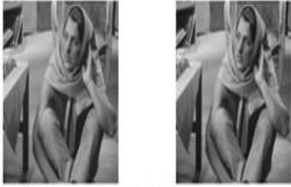
Fig11The original image (Left) and the watermarked image with 16298 byte hidden data and 34.04dB PSNR (Right)
