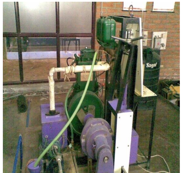
Fig.3.1 Single cylinder 4-stroke Diesel
